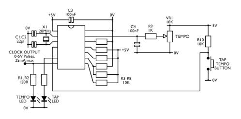
and the 'Next multiplier' input (tied high). The main LFO output isn't used. Tempo can be set either by the Tempo knob VRI or by tapping the button.
