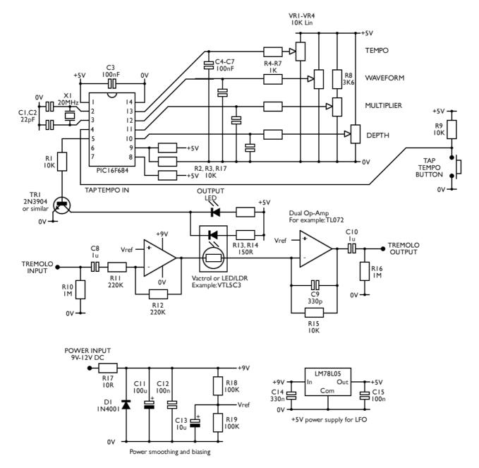
This example circuit shows a complete tremolo effect based on the tap tempo LFO. The tremolo audio path is a clean, simple design based on the classic Tremulus Lune. Thanks to Mike for his work designing this with my original PIC VCLFO.
