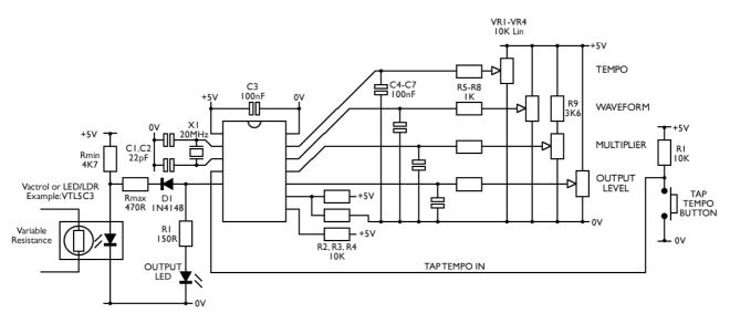
Rmin and Rmax control the minimum and maximum brightness of the LED. Rmin sets the current through the LED when the LFO output is at its lowest level. When the LFO output is at its highest level, the voltage on pin 5 is +5V, so Rmin and Rmax are effectively in parallel. The example VTL5C3 vactrol gives a variable resistance from 60K to 3K3 with the values given.
