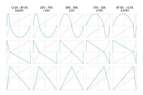
The top row shows the effect of the WAVE DISTORT CV on the SINE wave, whilst the following rows show the effect on the RAMP DOWN and TRIANGLE waveforms. Other waves (excepting RANDOM) are affected similarly.
