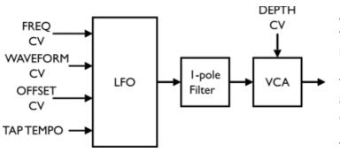
The STOMPLFO chip can produce eight waveforms, including two random waves. The basic LFO frequency is controlled by FREQ CV.
