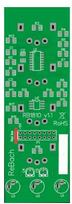
Connect the power cable with the red band facing to the left side of the module (rear view)
