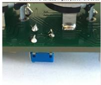
Place and solder the trimmers first before placing the potentiometers
