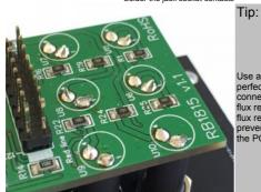
Use a little flux for a perfect solder connection (remove flux residues with flux remover to prevent damage to the PCB!
