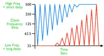
Blue:Top-down, Decreasing from max to min Depth Red: Bottom-up, Increasing from min to max Depth The Depth control introduces LFO modulation into the clock. The modulation is unipolar and can either be introduced from the "bottom up" - e.g. from the longest delay time towards the shortest, or "top down", from the shortest delay towards the longest.
